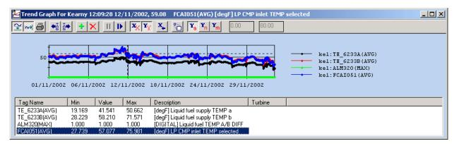
Trend graph showing liquid fuel temperatures A and B and selected liquid fuel temperature.
