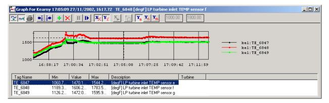
Data graph showing LP turbine inlet temperatures B, C & D.
